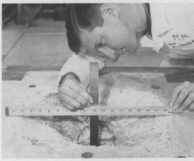
PHYSICAL DIMENSIONS of the model crater are carefully measured by M. R. Zimmerman. Results of the research study may have applications in the Plowshare program, peaceful atomic energy uses.
